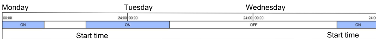
Figure 13: If an ON-time runs past midnight on a day when the 24-hour clock is not active, the function will remain ON until the time has elapsed.
