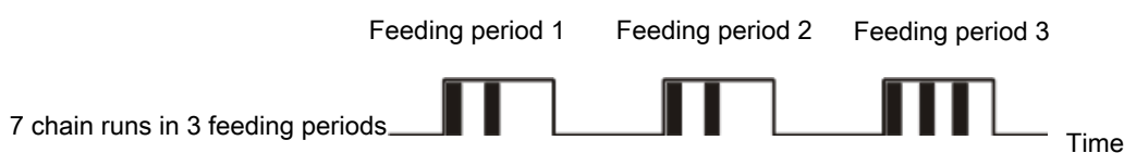
Figure 8: Chain feeding: Example 1: Distribution of number of chain runs The number of chain runs is distributed equally between the number of starts. Excess chain runs are distributed from the last start.
